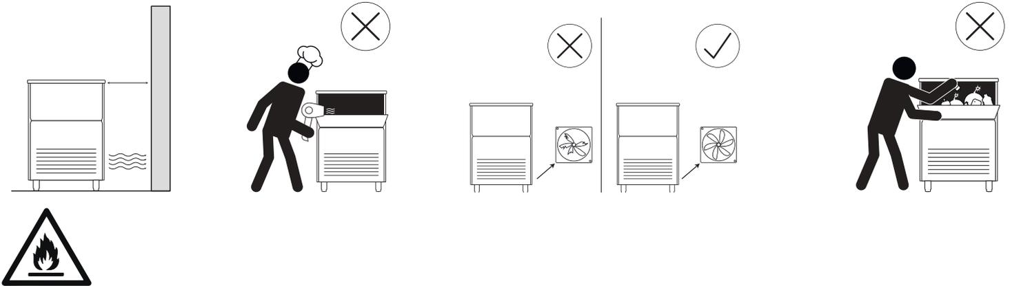
EN. In case of refrigerant leakage:
